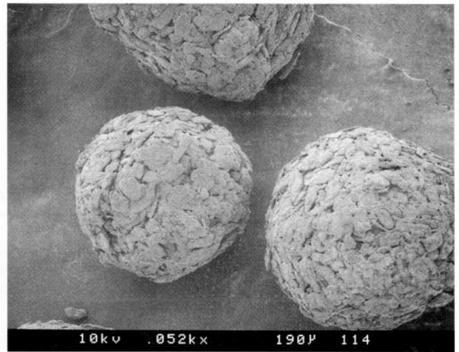
Fig. 3 d) AGT-processor: "Wet" processing (agglomeration of dry powder feed, dia. approx. 1 – 2 mm)
